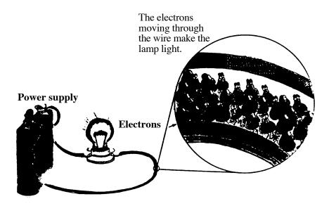
In certain substances, e.g., metal wire, electrons can be made to move easily by applying a power supply. Substances in which electrons move easily are called conductors.
