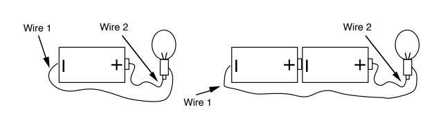
8. In this picture, the circuit is incomplete. This small gap will stop the current flow and the bulb will not light. Experiment with some of the materials in your baggy bag and see which object can be use to complete the circuit and light the bulb. The objects that help you to light the bulb are called conductors and the objects that don't help to light the bulb are called insulators. Use the chart to record your observations.
