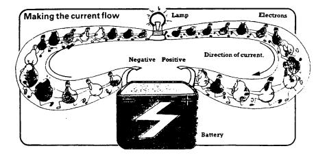
A battery is a power supply. It has two terminals. One terminal has a positive charge and the other has a negative charge. Electrons also have a negative charge. When wire is connected to each of the terminals, the electrons in the wire are repelled by the negative terminal and attracted to the positive. This causes the electrons to move through the wire and form an electric current.
